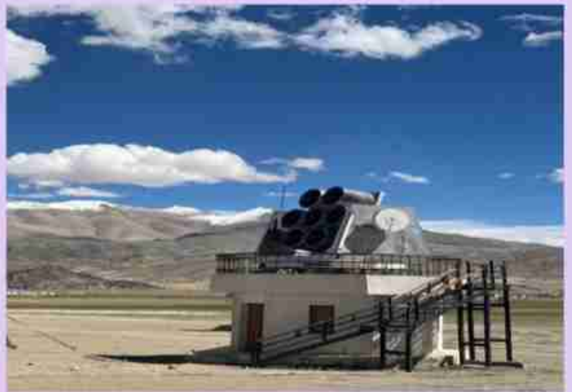
The High Altitude Gamma Ray (HAGAR) Telescope used for detecting high-energy cosmic rays.
